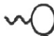
Fig. 9.2—Different types of surfactant structures. A hydrophobe is lipophilic and usually nonpolar. A hydrophile is lipophobic and usually polar. Molecular structure is often represented generically by the tadpole, with the tail being nonpolar and the head polar.
